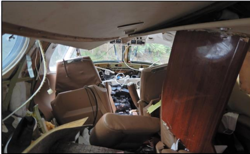
Figure 22 - Extent of damage inside the aircraft.
