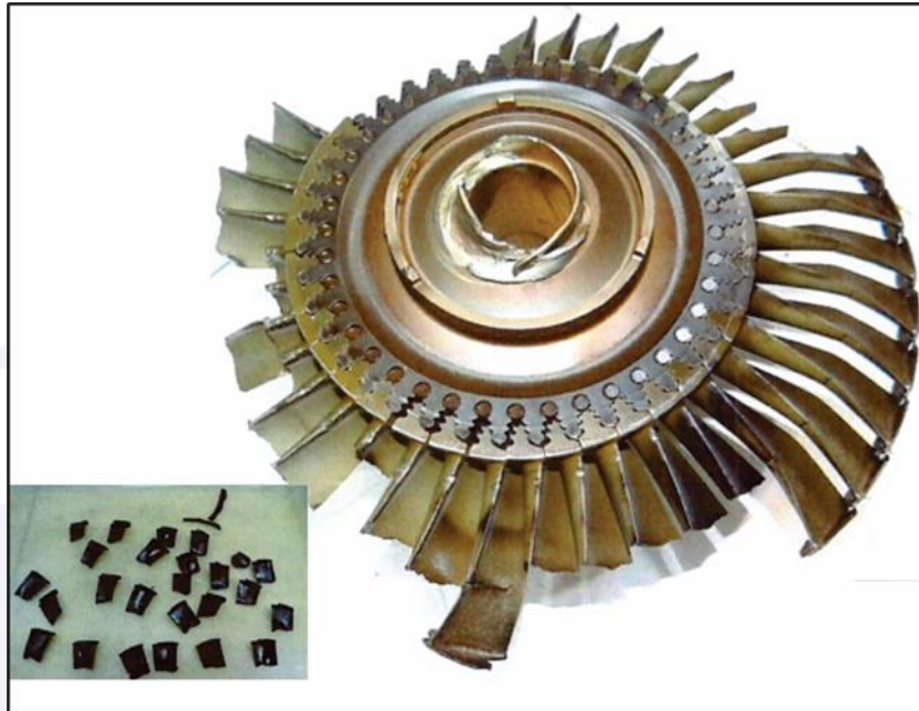
Figure 30 - Front view of the left engine power turbine rotor and part of the blades that were recovered.
