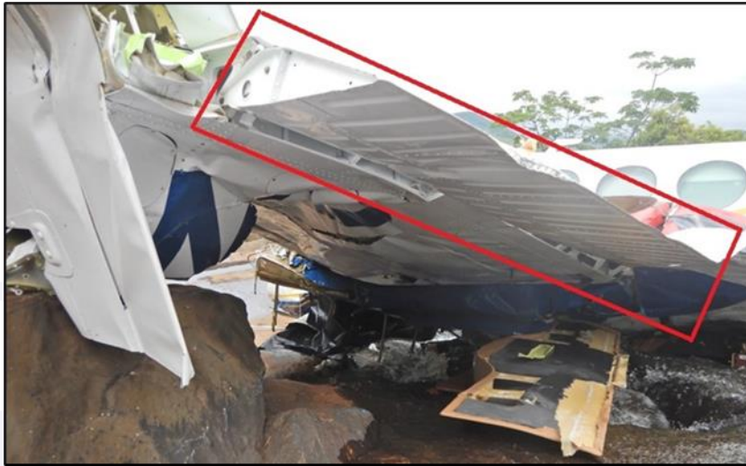
Figure 20 – Left-wing flap position after impact with the ground.
