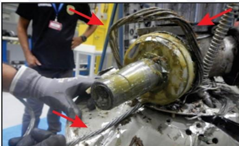
Figure 37 - Lightning arrester cable wrapped around the left engine propeller shaft, indicated by red arrows.
