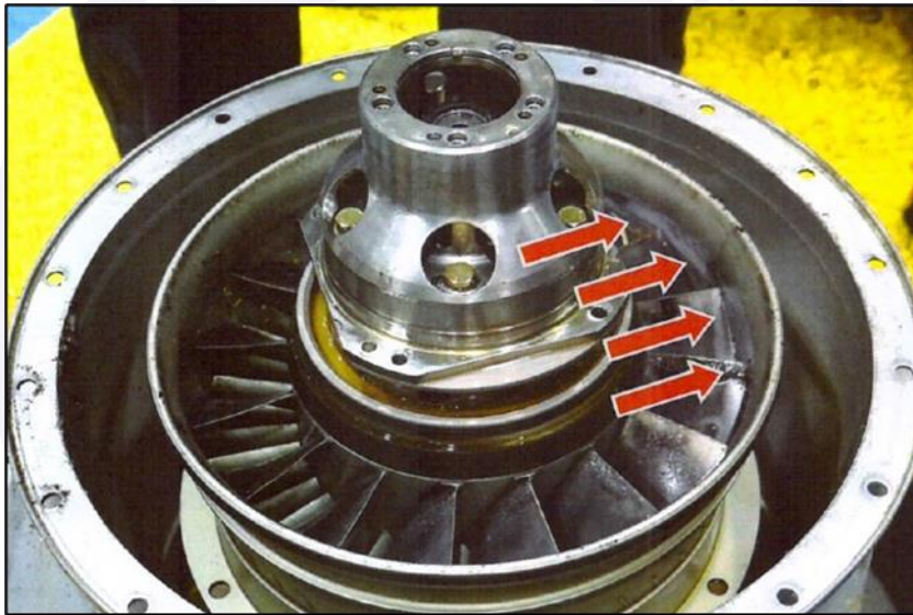
Figure 27 – View of the rotor of the first stage of the left engine compressor with rubbing marks observed on the housing.
