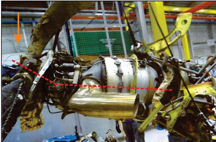
Figure 26 - View of the left side of the left engine without fairing. The dashed line projects the engine's longitudinal axis. The arrow indicates the cable wrapped around the propeller hub.
