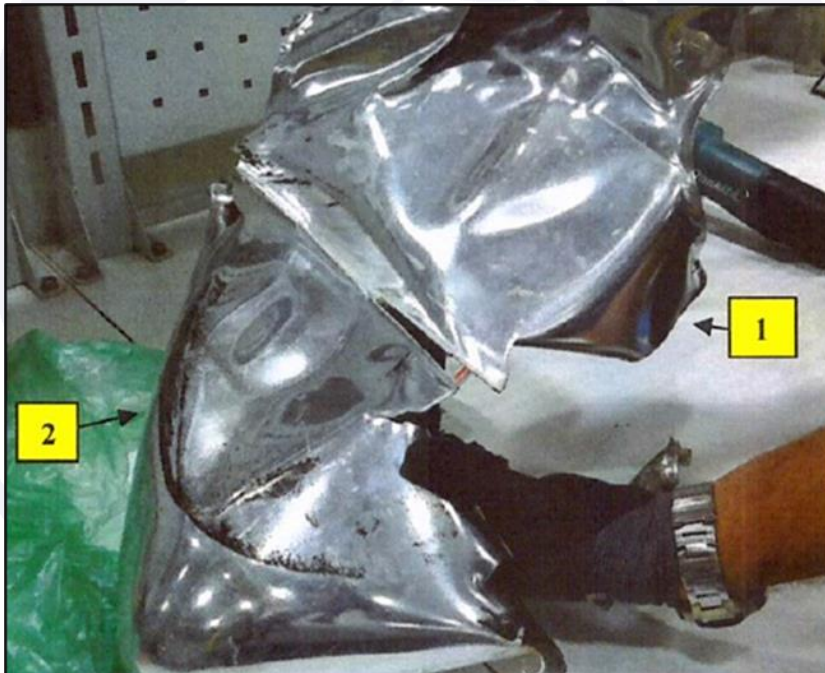
Figure 33 - Impact marks on the left engine spinner.
