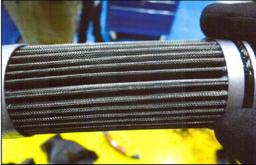
Figure 32 - Left engine oil filter without abnormalities.
