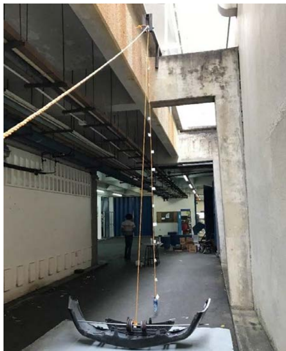
Figure 2: Image of simulated accident testing setup
