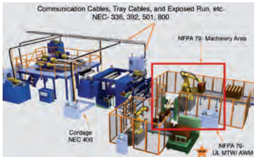
The diagram illustrates key NEC® and NFPA regulatory codes for an industrial plant manufacturing floor. Each code calls out permissible cables. 'NEC®' is a registered trademark of the National Fire Protection Association.
