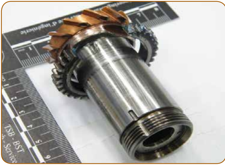
Failed gear on the torque sensor shaft
