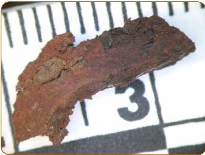
Debris found in fuel pump nozzle (ruler scale is cm)
