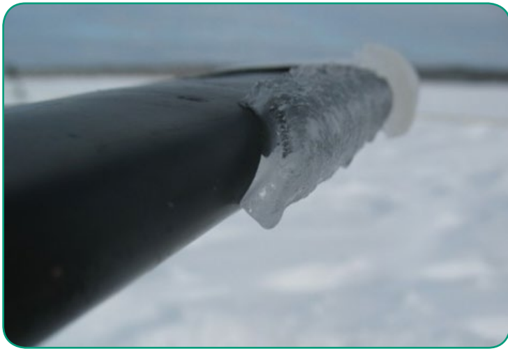
Photo 4. Ice on the horizontal stabilizer leading edge
