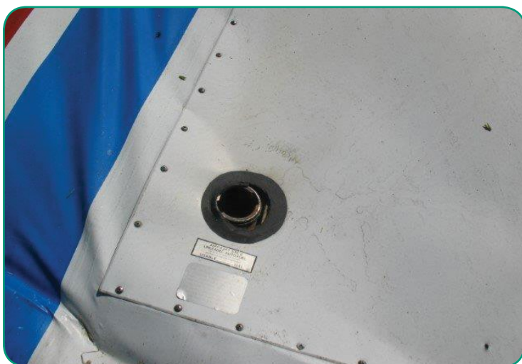
Both fuel caps were missing and could not be found.
