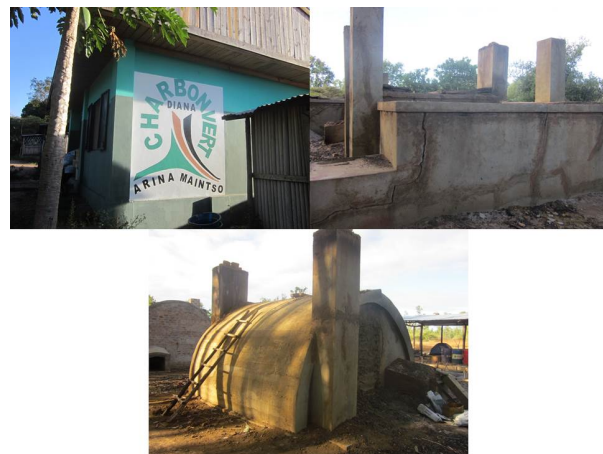
Fig. 6. Fuelwood interventions beyond the plantation implemented by GIZ PGM-E: (Clockwise from top left): Rural “Green Charcoal” supply depot; an older rectangular model of improved charcoal kiln, which cracked after a few firings; and the most recent dome-shaped improved kiln, which has withstood firings so far.
