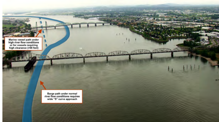
Photo: Marine vessel path on the Columbia River Source: Washington State Department of Transportation
