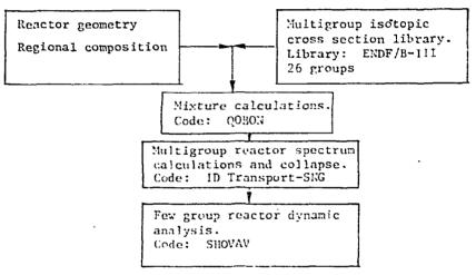
By using the above scheme, which was implemented on the IBM 370/165 computer, it is now possible to use ENDF/B-III data for the dynamic analysis of fast reactor systems.
