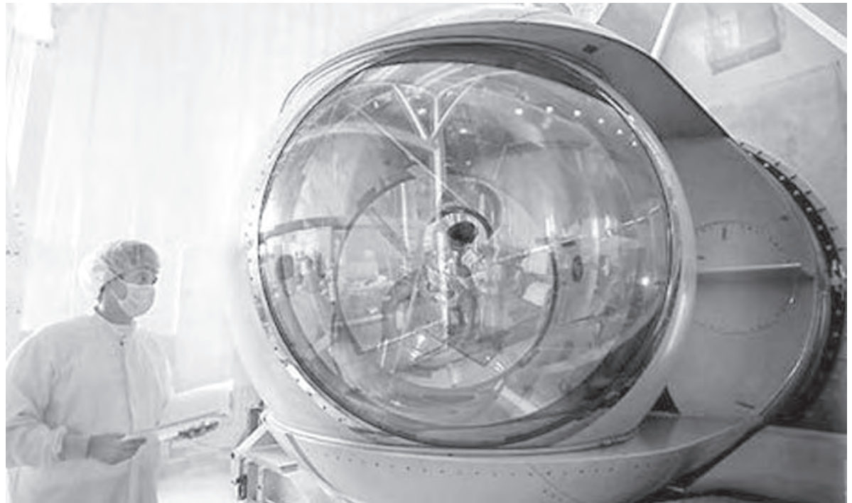
A technician examines the Airborne Laser nose turret, and the mirror which reflects the laser.
