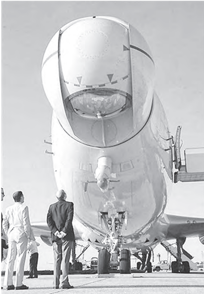
Inspection of the nose turret (open) of the Airborne Laser aircraft.
