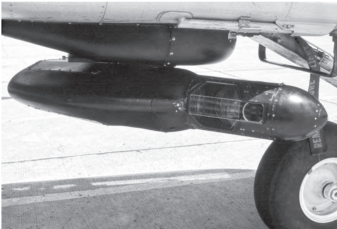
The PAVE SPOT turret. (Photo courtesy of Rick Atchison.)
