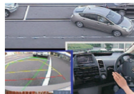
Intelligent Parking Assist and control board
