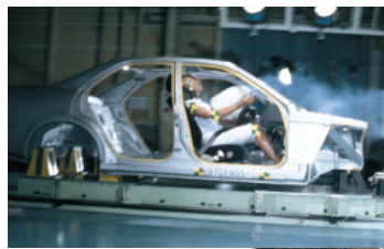
Sled-testing equipment that conforms to the latest regulations recreates both low- and high-speed crashes.
