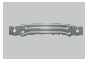
Bumper reinforcement employing die quench process
