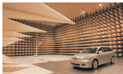
Anechoic chamber which evaluates the influence of electromagnetic waves on electronic devices (Fujioka)
