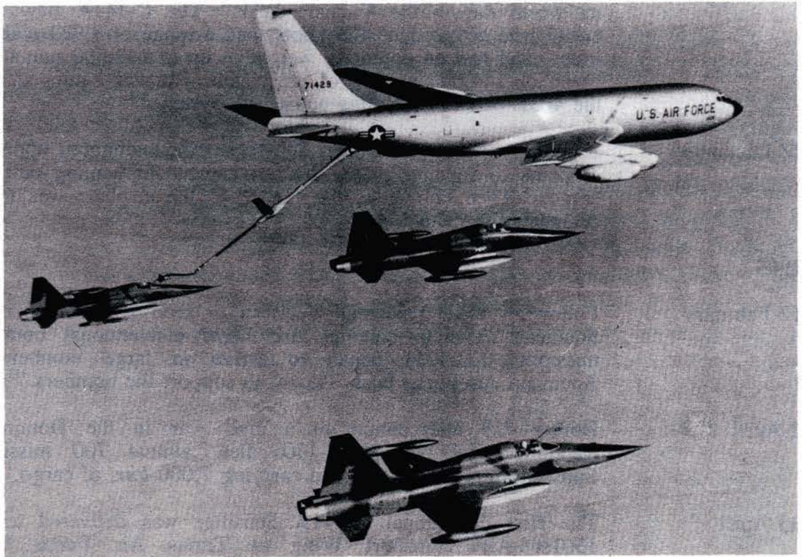
KC-135 Stratotanker involvement in the Vietnam War began in June 1964 and continued until August 1973. In 1965, KC-135s fueled experimental F-5Cs, which were F-5As modified to combat configuration with the addition of armor plate and other enhancements, on their way to Southeast Asia. (Northrop Corporation photo)
