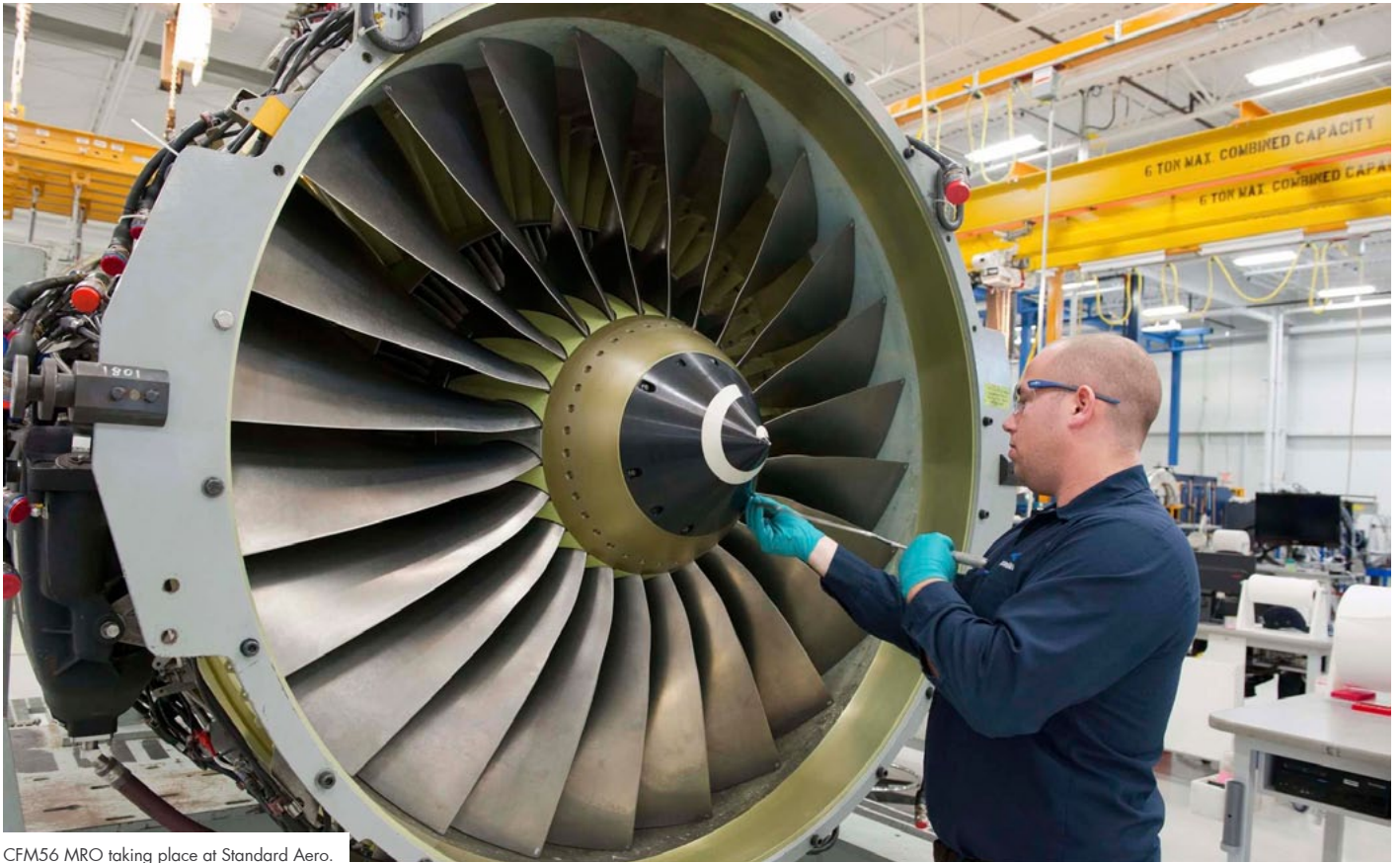
CFM56 MRO taking place at Standard Aero.
