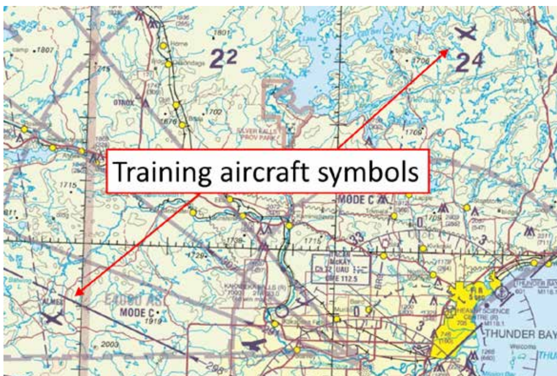
Figure 6. Training aircraft symbols on a visual flight rules (VFR) navigation chart (VNC) (Source: NAV CANADA, with TSB annotations)
