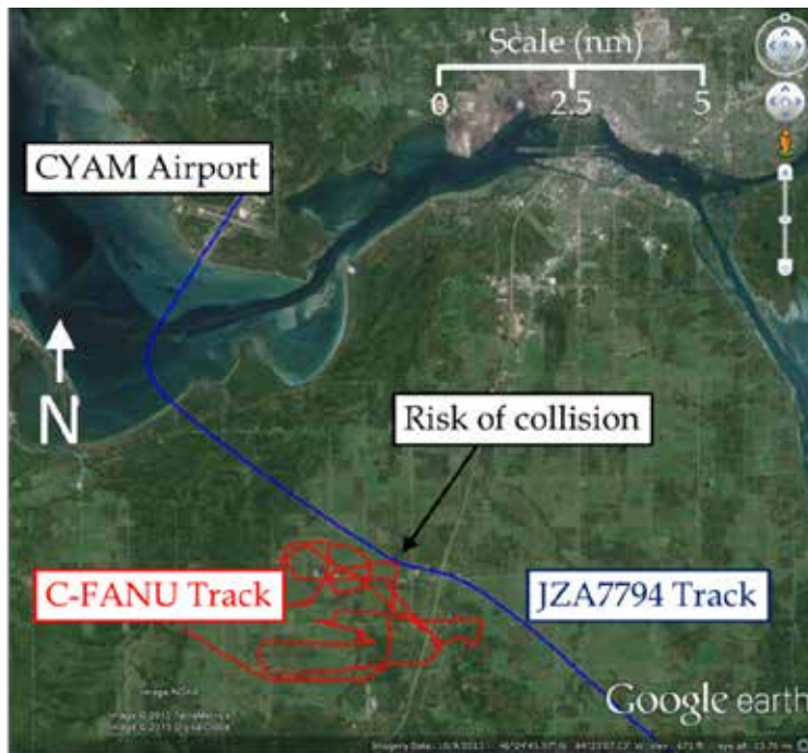
Figure 1. Depiction of the aircraft tracks leading to the risk of collision (Source: Google Earth, with TSB annotations)
