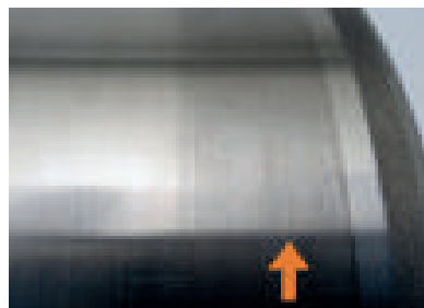
Figure 2 Adhesion occurs in equipment operating in the mixed and boundary lubrication regimes due to insufficient lube supply, inadequate viscosity, incorrect internal clearances, incorrect installation or misalignment.
