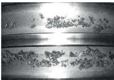
Figure 1 Fatigue spalling on the raceway
