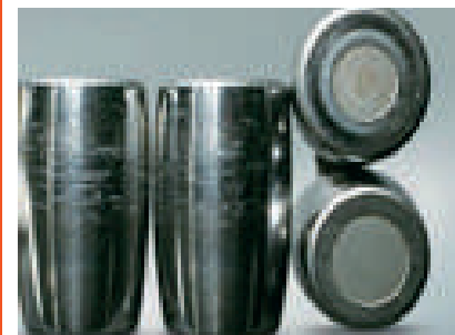
Figure 3 Abrasive wear is the result of inadequate lubrication or the ingress of foreign particles.
