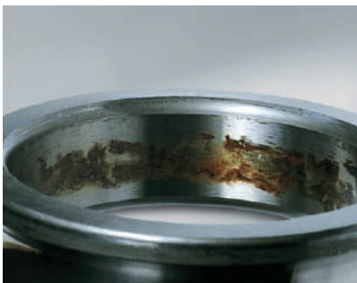
Figure 5 Fretting corrosion occurs in fit interfaces that are transmitting loads under oscillating contact surface micromovements.
