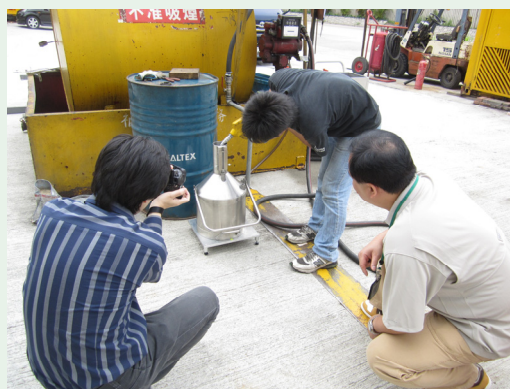
An officer of the Department and a Government Chemist checked the accuracy of a fuel dispenser at a fuel refilling station.
