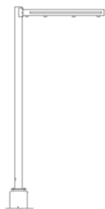
Single-Arm Cantilever Structure
