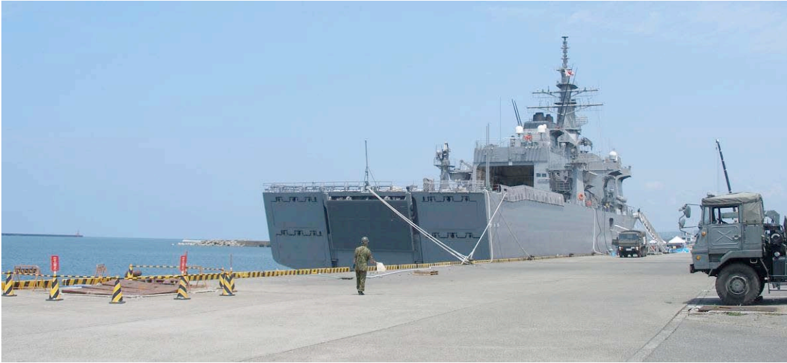
Figure 11.4: SDF ship at Kashiwazaki City port, July 27. SDF used desalination systems aboard ships to supply emergency water while local water systems were repaired.
