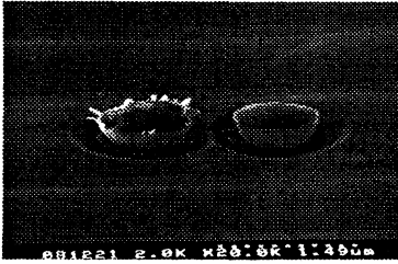
FIGURE 3. Via sidewall polymer removal pre- & post-vapor HF cleaning
