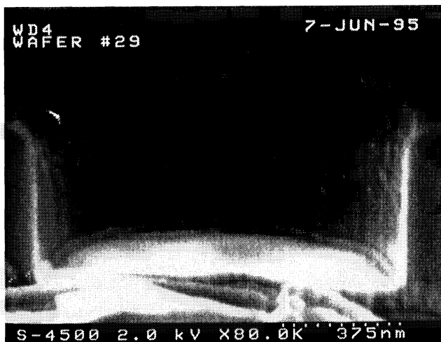
Figure 1 (Top): Via with heavy sidewall polymer and TiN undercut.
