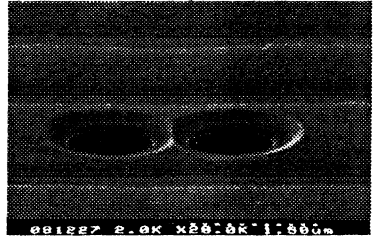
FIGURE 3. Via sidewall polymer removal pre- & post-vapor HF cleaning
