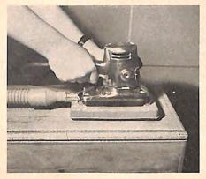
Orbital-action sander with a plastic skirt and hose that connects to a vacuum cleaner insures dustless sanding. This type of sander can be moved across as well as with the grain of your work.
