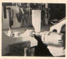
This "driver"-type drill has a speed of 3,200 rpm—enough to do fast sanding with drum (as shown) or with sanding disk. It also has plenty of power for orbital sanding, jigsawing, hedge-trimming.
