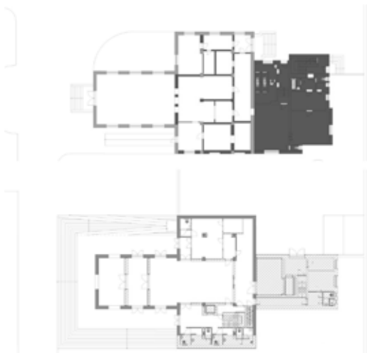
Fig. 6 Drawing of the original state designating the demolished parts (upper figure), drawing of the proposed new construction of mourning hall (bottom figure), Ostrava - Vítkovice, Daniela Rejmanová Venusová [5]
