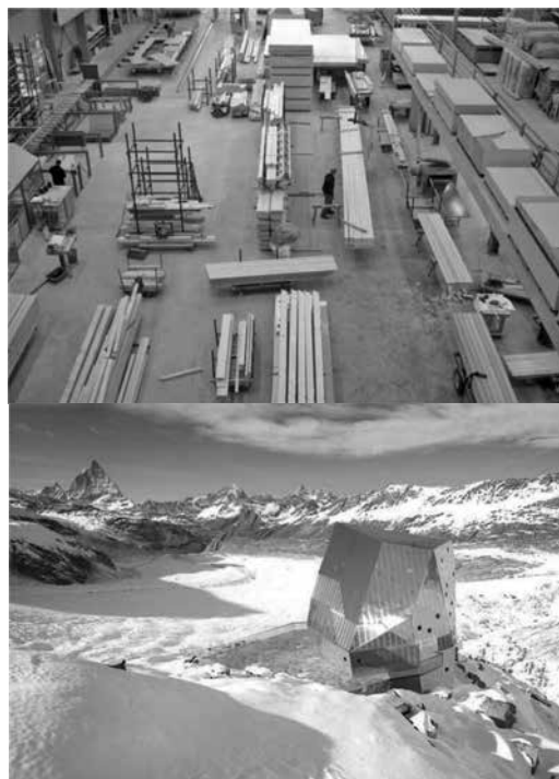
Fig. 2.,3.: The individual parts were digitally proposed by the computer and precisely manufactured in the factory. View of the Monte Rosa cottage in the Swiss Alps. (Source: L. Hovestadt: Beyond the Grid-Architecture and Information Technology, Birkhäuser Verlag, Basel, 2010, p. 155.)
