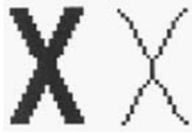
Figure 3. An example of necking, where the topological relationships of the binary data and skeletonised data have been altered.
