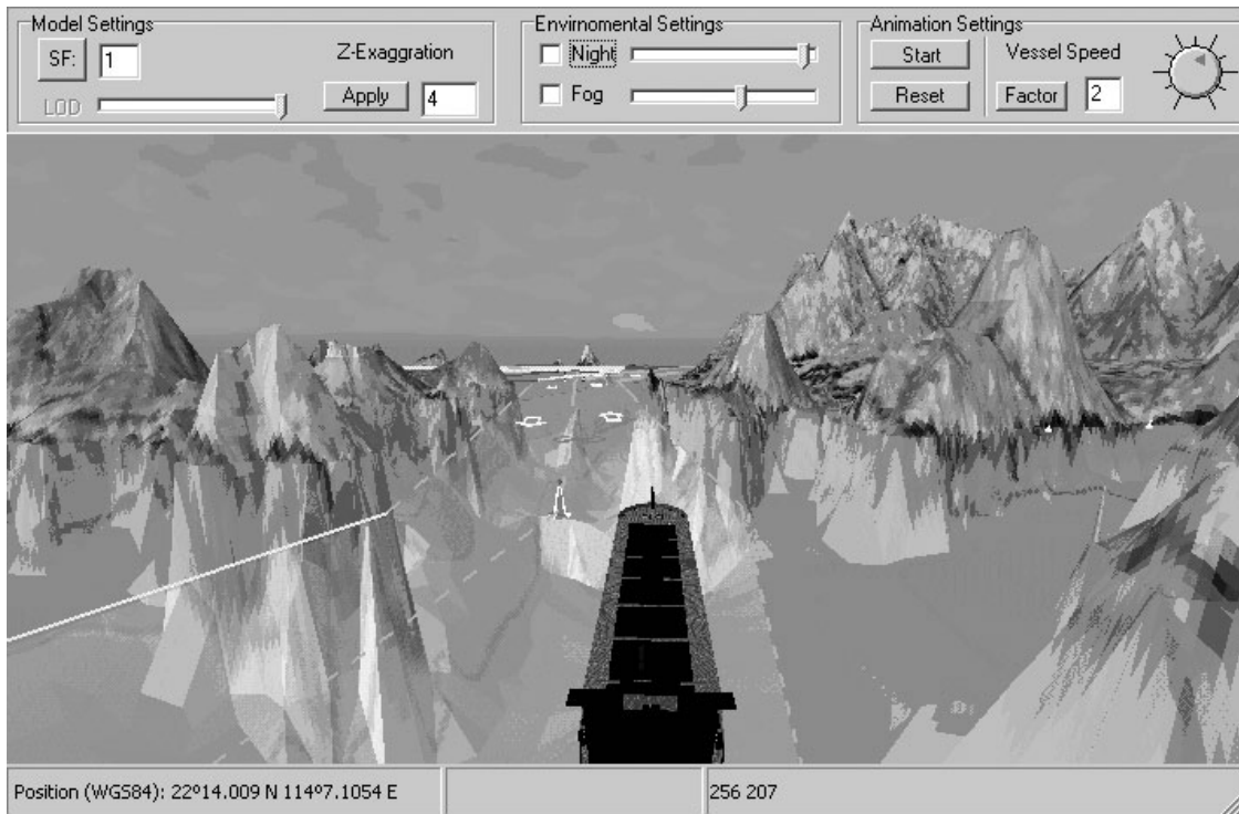
Figure 4. Scene in navigational mode. When animation mode is activated, the viewpoint will follow the movement of the ship model
