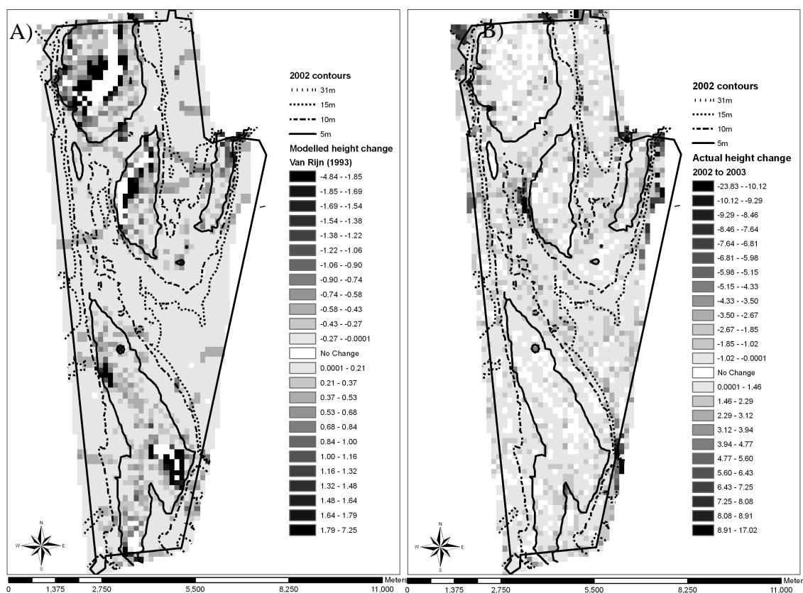
Figure 2: Predicted and measured seabed height change for the validation area between 2002 and 2003 at 150m resolution, height change is in metres. A) Prediction using the Van Rijn (1993) formula and rock case distribution and B) Measured difference.
