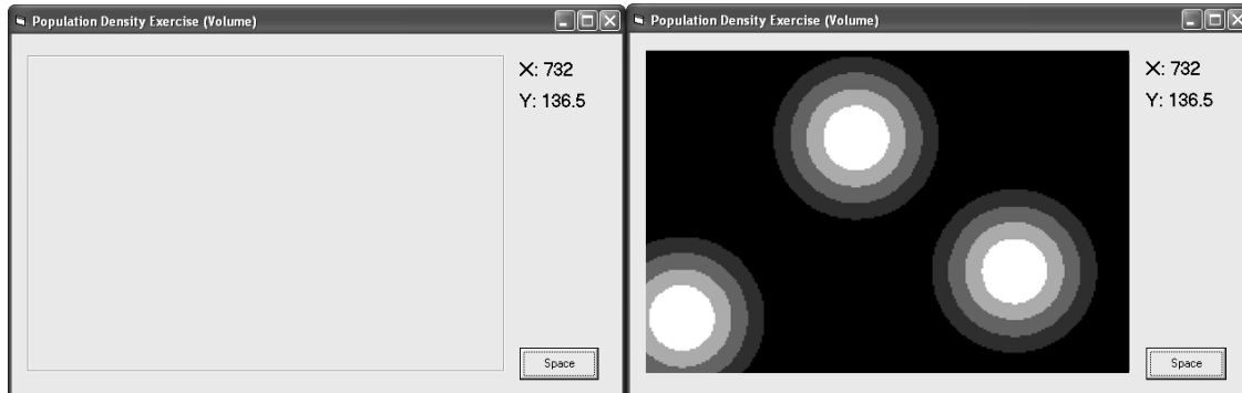
Figure 2. The Population Density Exercise shows the blank screen to the left shown to the user, and asks them to locate the 3 high volume (or tempo) locations. The screen to the right (not visible to the user) shows the variation in sounds played by the computer when the mouse is moved over that section, with a higher volume (or tempo) illustrated by the lighter colours.
