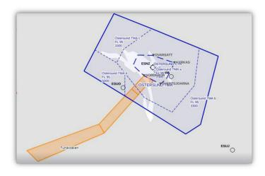
Flying in a restricted area is a solution that allows for Aviant to fly BVLOS within uncontrolled airspace. It is however limiting for the other operators to use the airspace freely. As the other operators normally fly during daylight hours only, Aviant decided to operate at night time.
