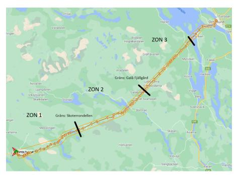
Evaluation of 4G coverage was the focus of the initial tests. The full path was divided into 3 different zones that were tested individually. Surprisingly, there was only one area that was beyond the tolerance, near Grundsjön, Härjedalen. As 4G reception increases with altitude in proximity to mountains, increasing the altitude by 80 meters was sufficient to solve this problem.
