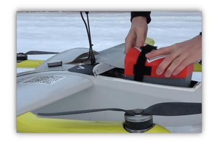
Initially, insulation was difficult due to temperature drops near the payload, but it was solved by using proper materials. A blood cargo box was made for the drone in the lab in Norway, but mostly the blood was transported in simpler styrofoam boxes. A handful of times, one blood tube was additionally transported by the regular road transport, so that the analysis could be compared by the lab in Östersunds Hospital.
