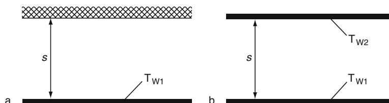
G2. Fig. 3. Boundary conditions for heat transfer in a parallel plate duct (in an annular gap for the case of (d_i/d_o) = 1 ). Boundary condition (a): Heat transferred from one side of the duct. Boundary condition (b): Heat transferred at both sides of the duct, each at the same wall temperature T_{w1} = T_{w2} .
