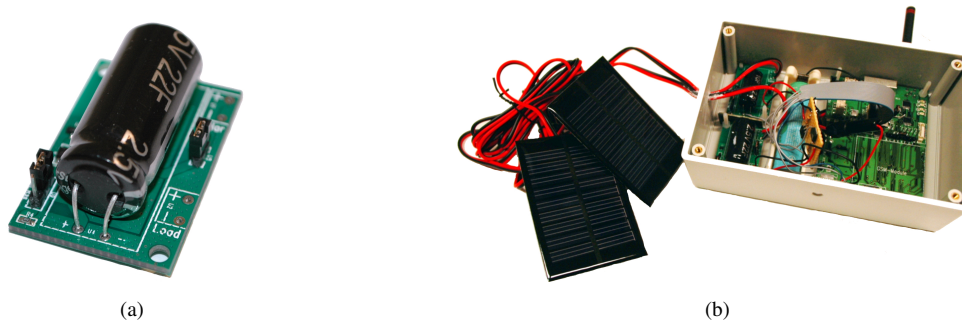
Figure 9. Implementation of the deployment system - (a) Direct coupling harvester circuit board; (b) Complete system integration
