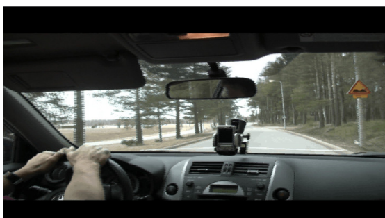
Figure 5. Test system set-up in vehicle. Mobile phone installed in car dock in the middle.
