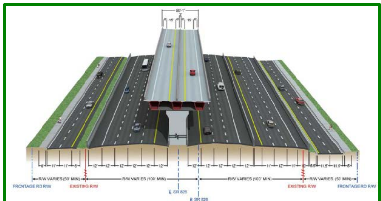
Proposed Typical Section – SR 826/Palmetto Expressway From NW 17 th Avenue to Golden Glades Interchange
