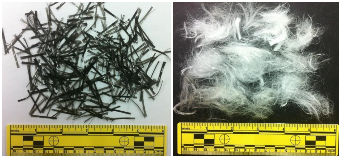
Figure 22. Polypropylene monofilament (left) and polypropylene defibrillated fibers (right)
