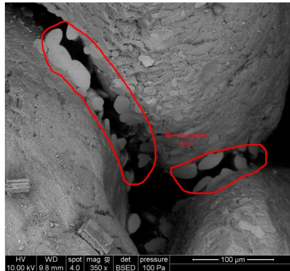
Figure 23. SEM image from bio-treatment of silica sands at ISU (350x) (Li, 2012)
