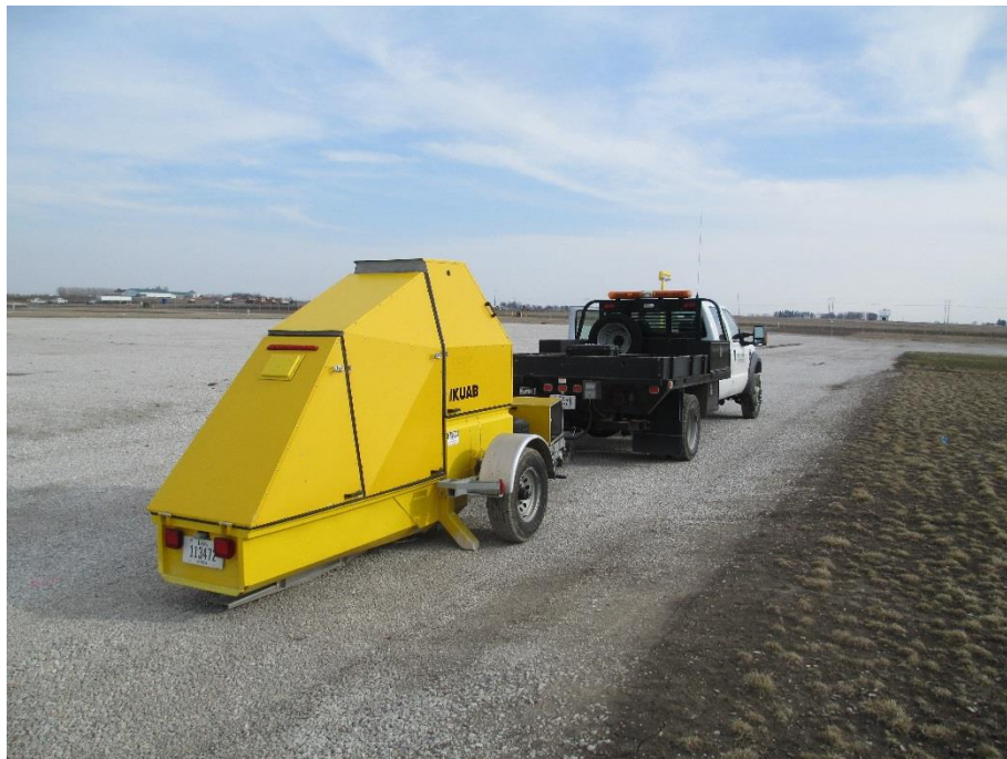
Figure 29. ISU-Kuab Falling weight deflectometer
