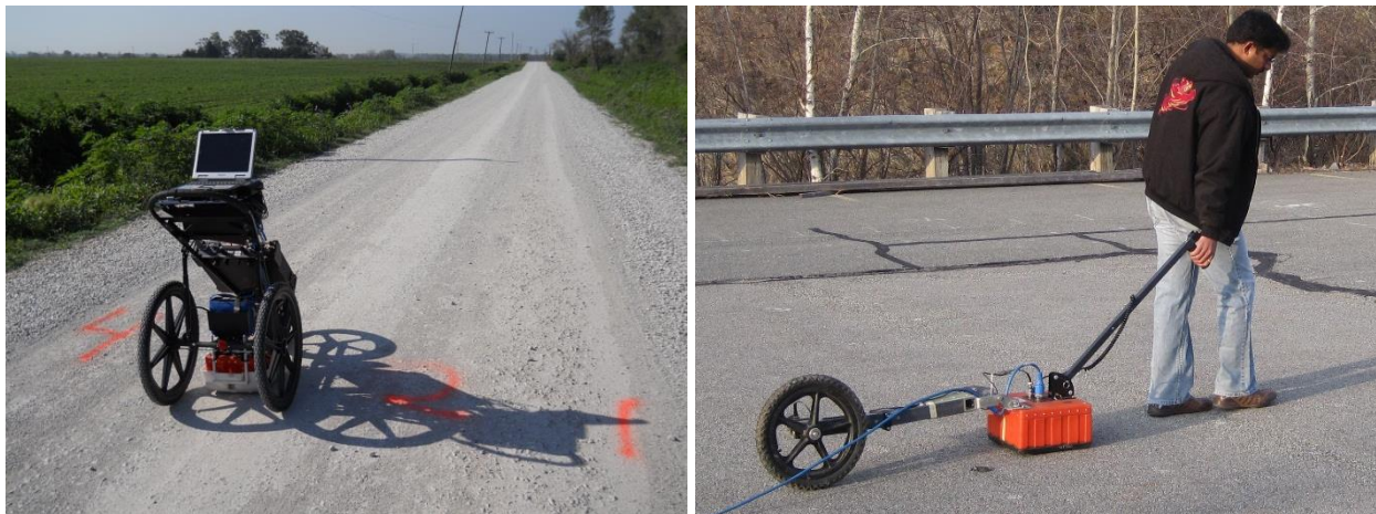
Figure 31. ISU-GPR scanning using ground-coupled antennas
