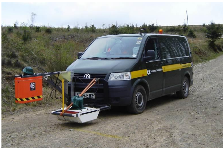
Figure 32. Air borne GPR survey vehicle used for condition assessment on ROADEX projects in Europe (Drake 2012)
