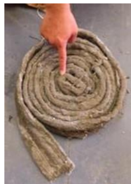
Fig. 3.7. Plastic drain that was installed 50 years ago without documenting location and prevented jet grouting for recent construction.
