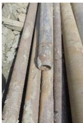
Fig. 3.27. Example of poorly-maintained field investigation equipment.
