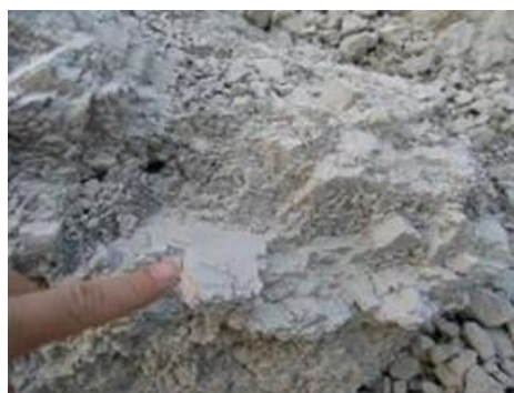
Fig. 6.2. Rock powder mashed by collision between Indian subcontinent and Eurasia, resulting in many slope instabilities (Himalayan front in Nepal).
