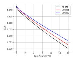
Figure 2. Deterioration of the effective multiplication factor with various depletion schemes
