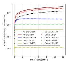
Figure 4. The atomic density of FPs in fuel salt of nopro and Degas1.
