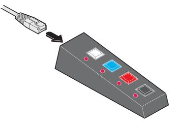
2 Connect the other end of the cable to the **OPTIONS** port on the rear panel of the switch.
