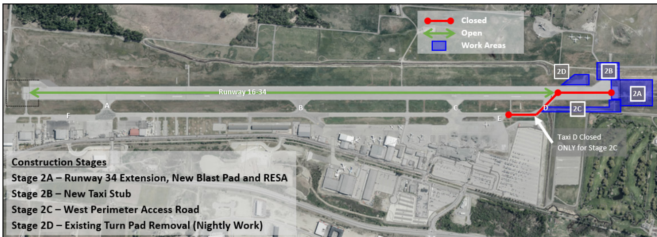
Figure 1: Stage 2 Construction Limit and Runway Availability
