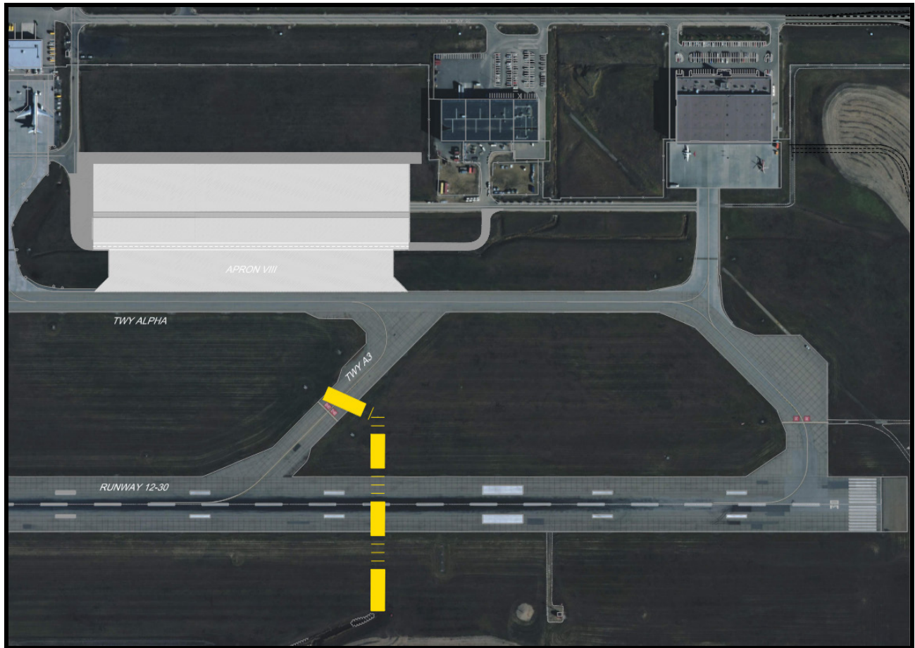
Figure 22: Runway 12–30 Stormwater System Upgrade Construction Limits
