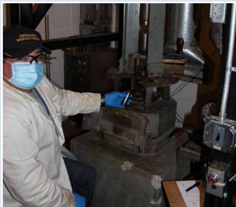
Dissection and Machining Branch hazards testing technician Dick Jones prepares test samples on the Explosives Research Laboratory's impact machine. Hazards testing supports production, ordnance assessment and research programs. The data allows engineers and researchers to verify the relative sensitivity of their energetics when compared to defined standards.
