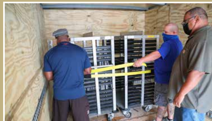
M Department employees Gerard Heard Jr. and John Shumpert participate in new eTrack training, overseen by M21 employee and Forklift Training Course instructor Floyd Proctor, Sept. 2. eTrack is a new cargo restraint system designed to better secure items during transportation moves.
