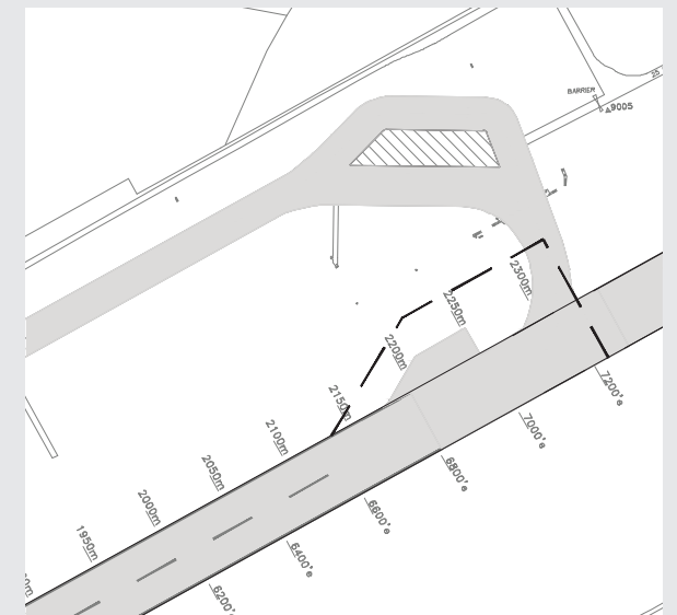
Figure 19 – Potential Runway Turning Area
