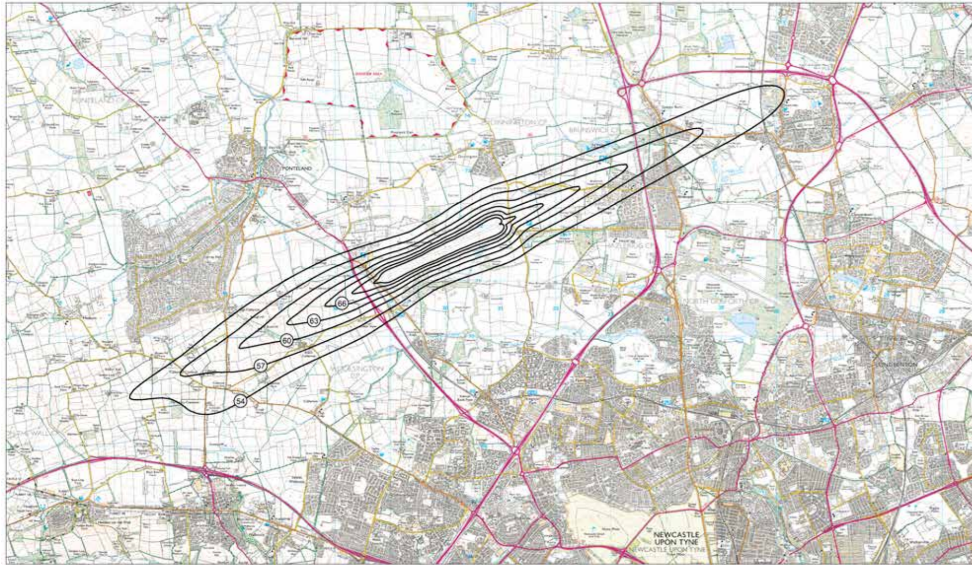
NEWCASTLE INTERNATIONAL AIRPORT 2016 Peak Summer Day L_{Aeq,16hr} 54-72 dB(A) Contours Modal Split 71% W / 29% E
