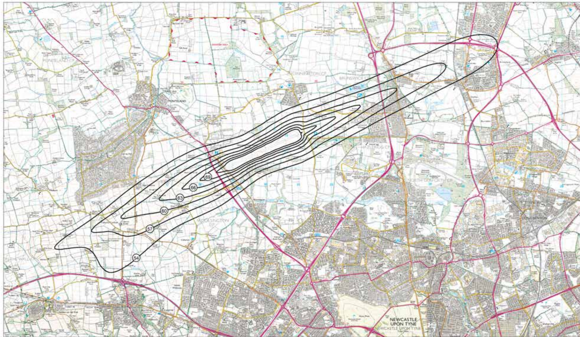
NEWCASTLE INTERNATIONAL AIRPORT 2025 Peak Summer Day L_{Aeq,16hr} 54-72 dB(A) Contours Modal Split 71% W / 29% E
