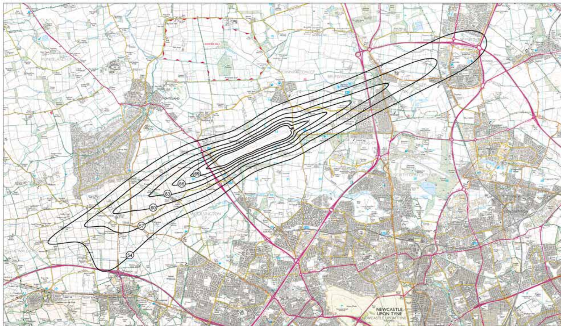
NEWCASTLE INTERNATIONAL AIRPORT 2030 Peak Summer Day L_{Aeq,16hr} 54-72 dB(A) Contours Modal Split 71% W / 29% E
