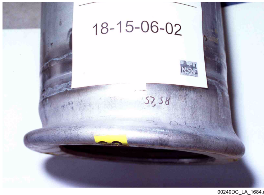
Figure 1.5.1-23. Deformed Shape of Standardized Canister for 30-ft Center-of-Gravity over Corner Drop (Lower End-Side View)
