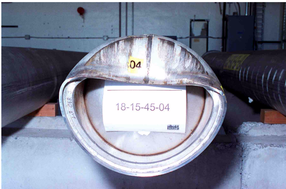
Figure 1.5.1-25. Deformed Shape of Standardized Canister for 45° Drop from 30 ft (Lower End-End View)
