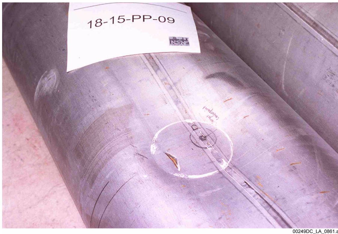
Figure 1.5.1-27. Deformed Shape of Standardized Canister for 40-in. Drop onto a 6-in. Post (Isometric View)
