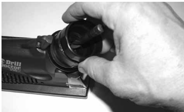
Top: The collet chuck has indexing fingers to clock the drill bit. Left, the collet chuck is rotated and the cams on its bottom cause it to rise and fall to provide back clearance for the cutting edges.
