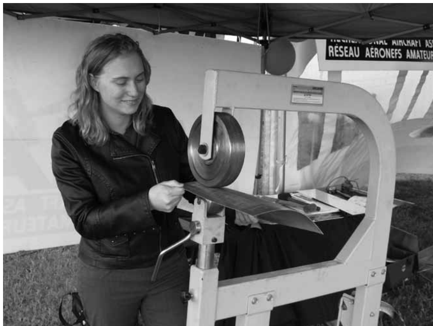
RAA Canada had a metalworking display at the Aircraft Spruce show in Brantford. Above, left Jacqueline Nusko of Wiarton was one of the attendees who learned the basics of the English Wheel. Top right, Member Len Halley demonstrated the use of the English Wheel to form aluminum. Right, RAA treasurer Wayne Hadath with his F-1 Rocket race plane was one of the featured acts at the Waterloo Airshow.
