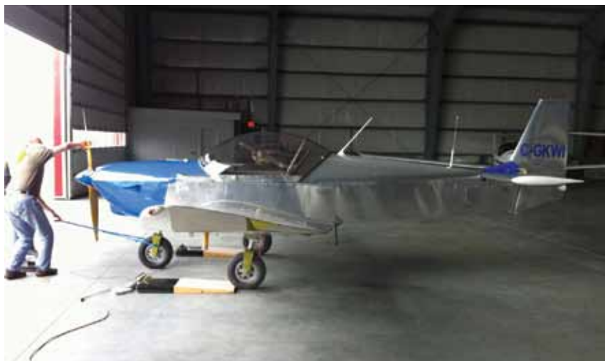
Members pull Peter Whittaker's Zenith 601 HDS onto the RAA scales in preparation for doing the weight and balance.
