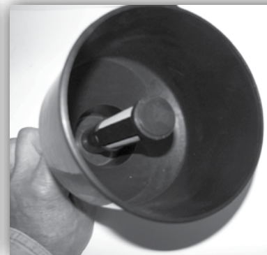
LEFT TO RIGHT: This is water and some swill that would not pass through the screen And here is the water back home in its bottle, with some fuel swill and debris to boot. The sump allows water to collect instead of blocking the mesh screen.
