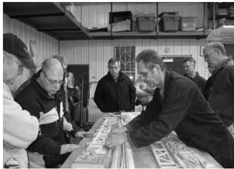
RAA Winnipeg, RAA Brandon, the Brandon Canadian Air Training Plan Museum and The Canadian Aviation Historical Society have been hard at work restoring their Tiger Moth. Here members learn the finer points of DeHavilland rib construction and installation.
