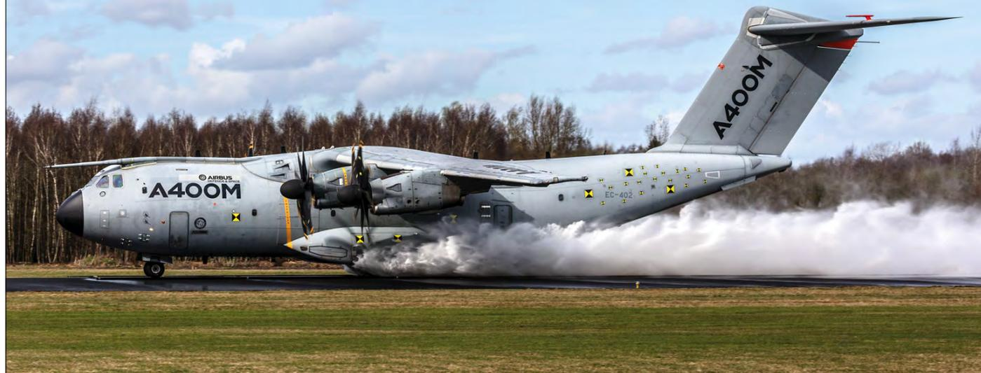
Only days before the dormant Twente Air Base was turned over to civilian control Airbus had contracted Dutch NLR for a couple of standing water runway tests. Prototype A400M EC-402 was used for the trials. (Twente, 21 March 2017, Pascal van Uffelen)
