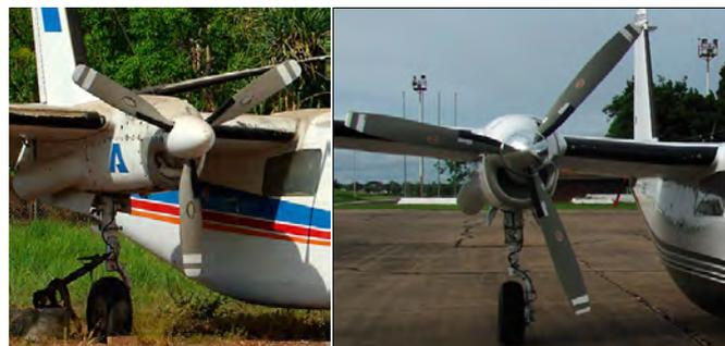
These two details show the difference between the early model Turbo Commanders and the later models, from 690 on. On the Commander 690 the engines are further from the fuselage, so that larger propellers can be used. As you can see the difference in prop diameter is significant.
