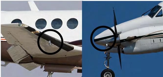
You can tell if the King Air 90 is an early model (90, A90, B90 or C90) by looking at the location of pitot tube: it is underneath the wing (left photo). Later models have it on each side of the nose.
