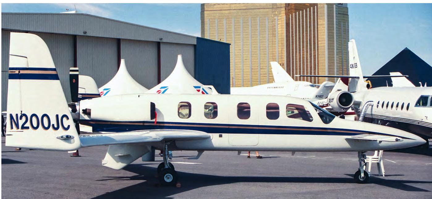
Just a few Jetcruzers were built before Advanced Aerodynamics & Structures Inc. (AASI) went bankrupt in 2002. It was a unique aircraft, being a single engine turboprop in canard configuration. N200JC was displayed at the NBAA convention in 1998. (Las Vegas-McCarran (NV), October 1998)
