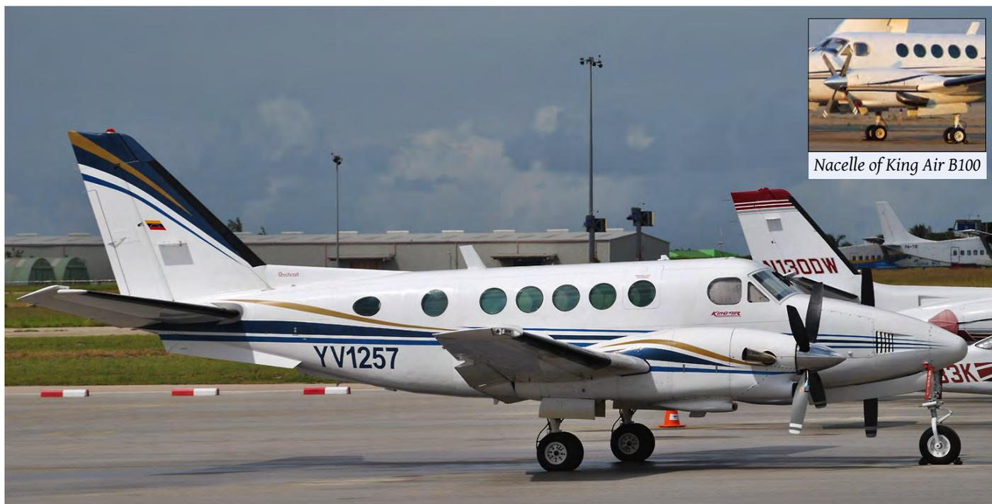
The Beech 100 is a stretched version of the Beech 90, which thus has more cabin windows. Also it has two wheels on each main landing gear. YV1257 is a Beech A100 and has four bladed props as a standard. In addition this particular aircraft has redesigned engine intakes, which more resemble those of the King Air C90A. The inset shows the nacelle of the King Air B100. Note the large exhaust pipe! (Aruba, 22 October 2010, Ruud Fopma)
