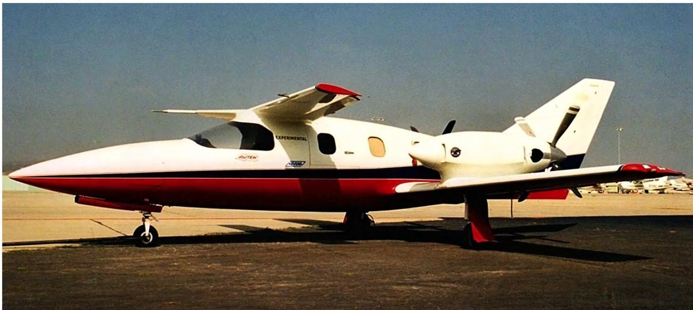
Many have tried to build futuristic looking aircraft, but many also failed finding a market. This applies to Avtek, which built a single proof-of-concept of the Avtek 400. Like the Beechcraft Starship it has a canard configuration, but the canard on top of the cockpit make it one of a kind. (Camarillo (CA), 19 October 2000, Peter Davis)
