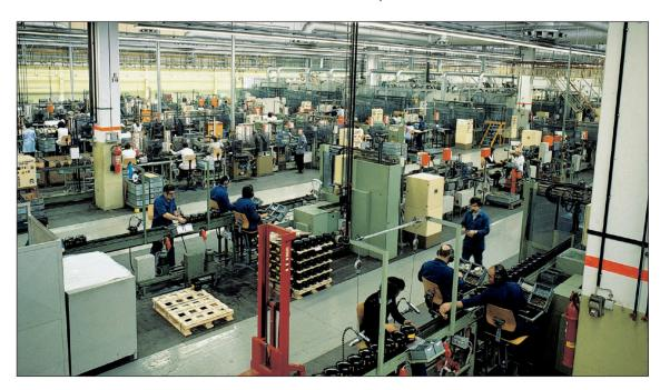
Assembly line in the compressor production.
