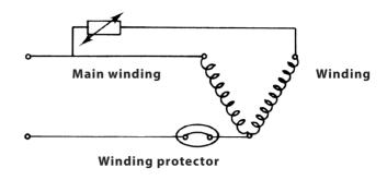
Wiring diagram with PTC and winding protector.
