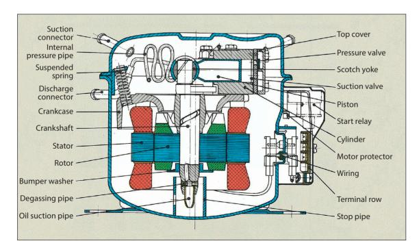
Cross-section of PW compressor.
