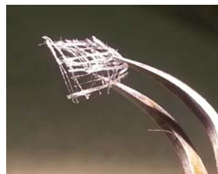
Figure 6: Multi-layered, wet-spun mesh of 1% wt/v alginate containing 20M cells/mL.
