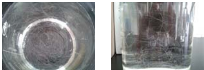
FIGURE 7. Dispersion after agitation of the one-step modified polypropylene fibers
