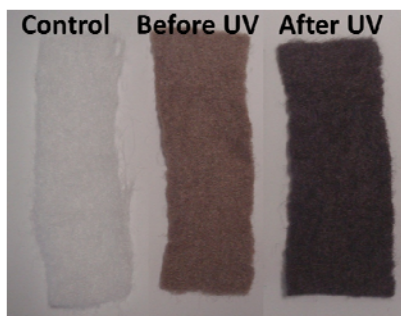
Figure 3. Optical images of polyester fabric, GO@ZnO functionalized polyester fabric before and after UV irradiation for 3 hours.
