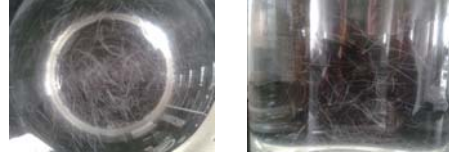
FIGURE 8. Dispersion after agitation of the two-step modified polypropylene fibers
