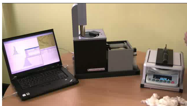
Figure 1. Cottonscope system (computer, data collection module unit including water tank and digital microscope, snippet preparer).
