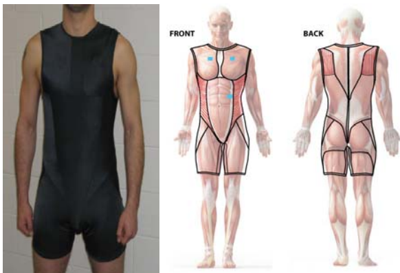
Figure 3. ECG monitoring garment with the componentized fabric panels. Striations show the gradient of the stretch orientation.
