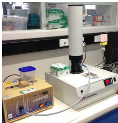
Figure 1 Lumipol 3 CL instrument modified to carry out PICL studies
