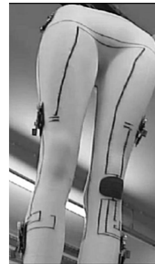
Figure 2 – Legging prototype made with a polyamide base yarn and silver yarn for communication and power lines.
