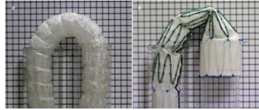
Figure 3: Bending behaviour comparison of stent-grafts. (a) Polymeric and (b) Zenith Flex® stent-graft subjected to 180° bending
