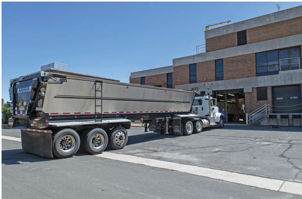
A semi-truck pulls into the dewatering building at the Drake Water Reclamation Facility to fill up with a load of biosolids. The trucks carry about 580 loads of biosolids per year to the ranch. One load covers 1.34 acres; the application rate is calculated at about 3 to 4 dry tons per acre.
