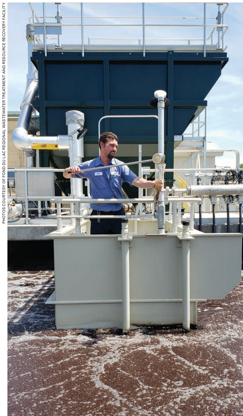
Standing on the internal settler over the anammox reactor, Mike Nolde, wastewater operator, pours a reactor sample into an Imhoff cone to check for granule quantity, size and color.
