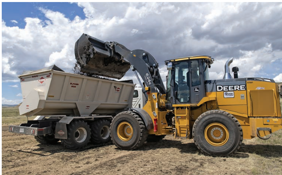
The Meadow Spring Ranch crew loads dried biosolids into a Kuhn Knight Slinger 8132 truck bed, preparing for distribution on the city's cattle ranch property.
