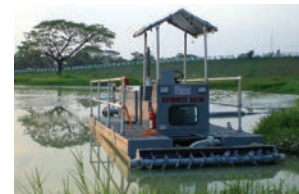
SD-110 Rotomite dredge from SRS Crisafulli System
