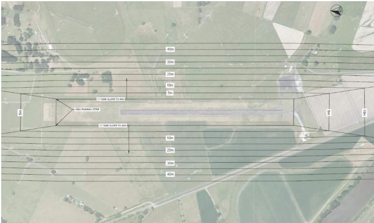
Image 9 – Obstacle Limitation Surfaces for Wairoa Airport (the contours show the maximum height limits for structures and vegetation).
