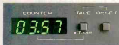
The real-time counter reads out the amount of tape left in meaningful minutes and seconds instead of meaningless inches.
