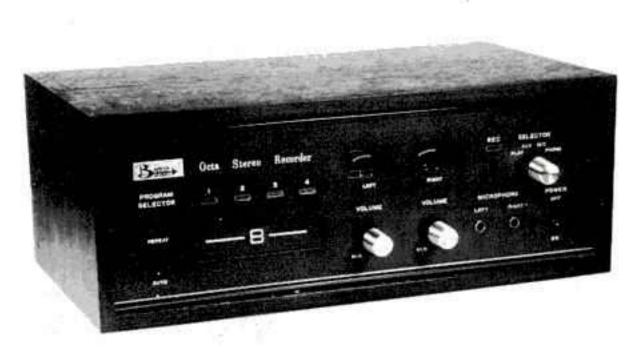
THE OCTA 8, an 8-track playback unit from California Auto Radio, features VU meters for left and right channels record level, record lock-out switch, channel change lock-out switch, balance and volume controls, microphone inputs and program selector.
