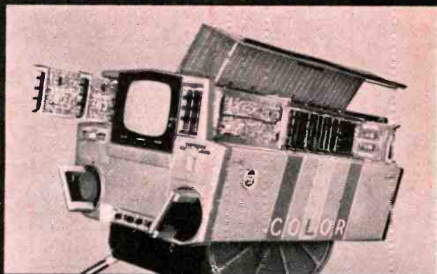
Transistorized modules afford easy servicing, are more reliable, and provide highest performance.
